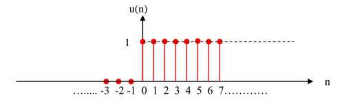
Unit step signal u(n) is the sum of a train of unit sample sequences
