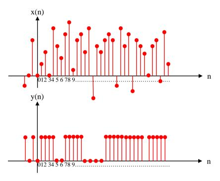
Amplitude restricted version of discrete time signals are called digital signals, for which the different number of amplitudes are restricted to finite number (Two). y(n) is a digital signal and all digital signals are discrete time signals. Digital signals can be obtained from discrete time signals by quantization mechanism.
